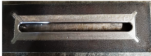
FIGURE 15. Image of the die after CNC machining processes.
